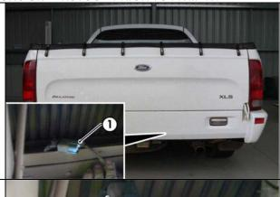
Connect the Trailer Harness Patch (P/N 100023-WL) connector (1) to the 8-way Breakout connector (2).
