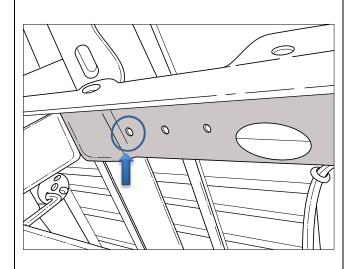
Loosely secure the Towbar Sidearms to the outside of the Chassis Rail using 2x M12 Bolts, Washers and Taped Plates on both sides of the vehicle.
