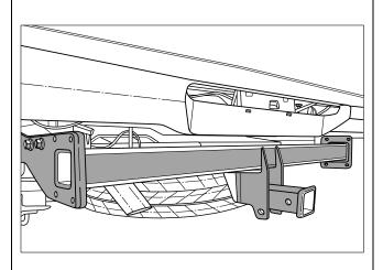
Align the Cover Plates to the outside of the sidearms. Secure the Cover plates to the sidearms and Towbar Centre with 4x M12 Bolts, Washers and Nuts.
