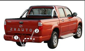
7. Connect the tail harness (tail length 1200mm) 8-way connector (1) to the trailer patch mating 8-way connector (2).
