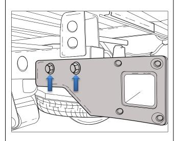
Loosely secure the vertical mounting points of the Sidearms using 2x M12 Bolts, Washers, one M12 long Taped Plate for the most rearward mounting point and an M12 Taped Plate for the most forward mounting point.
