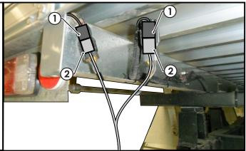
**3.** Route the trailer harness along the rear chassis towards the RHS of the vehicle.
