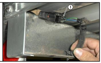
2. Disconnect the 6-way tail light connectors (1) and connect the trailer harness (100772-WL) connector (2) in between.
