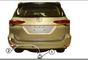
14. Route the trailer patch ORANGE power wire underneath the vehicle following the LHS chassis rail to the engine bay accessory fuse box. Keep harness routing clear of all moving parts, sharp edges or places of extreme heat. Appropriately secure the harness at 200mm intervals using cable ties (not supplied) after routing.
