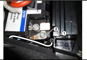
**14.** Remove the battery white plastic lid and secure the trailer patch power ring terminal (1) to the indicated vehicle positive terminal (2).
