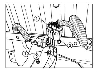
9. Using a tek screw (not supplied), secure the trailer patch ground ring terminal (1) to a suitable nearby location on the vehicle LHS frame rail (2).
