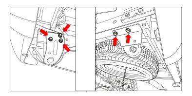
Loosely secure RH side arm to chassis rail with 2 x M12 bolts complete with 1 x washer per bolt on the inboard side of chassis rail and 4 x M12 bolts complete with 1 x washer per bolt to the underside of chassis.
