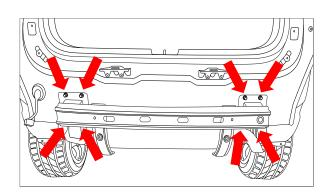
Enlarge the rear chassis rail mounting hole to accommodate a M12 bolt (Drill hole to 13mm). Deburr and apply an anti-corrosive coating to the exposed area.
