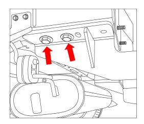
Secure the (drilled out) rear most hole position with 1 x M12 bolt complete with 1 x fitting plate, 2 x washers and 1 x nut. Ensure that the fitting plate is on the inside of the chassis rail.
