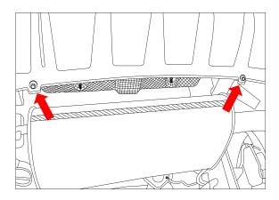
6. Peel away from the sides and remove bumper. Ensure to disconnect any wiring connectors from the main loom located on the LH side.
