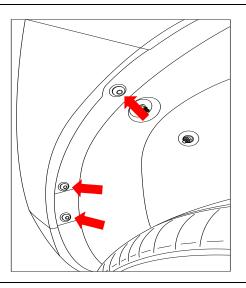
4. From under the vehicle, remove 1 x scrivet from the bumper.
