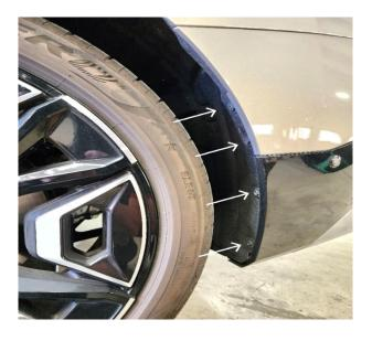
2. Peel back felt and remove plastic clip. Repeat for other side.
