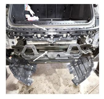
8. Remove impact beam via 4 nuts on each side.
