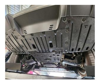
3. Remove all 10mm screws from underside of bumper and under body tray.
