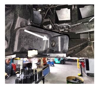
6. Remove bumper by peeling out from wheel arches and removing towards rear of vehicle.
