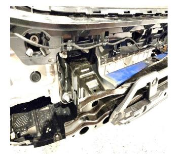
10. Using factory bumper cut template as a guide, measure from the inside edge. Use top and bottom of template as your height and cut 90mm into template. See picture below.
