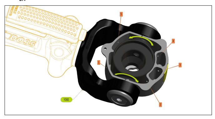
Flip over the yoke and feed the zip tie through the numbered holes in numerical order making sure that it goes over the visible side of the yoke pivot in order to hold down the bump cover as shown in the diagram. Pull tight and cut off excess. Test fit dust cover and locking mechanism for any interference.
