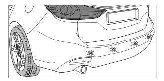
The PDC or SCBS-R system is not active while the parking brake is engaged.
