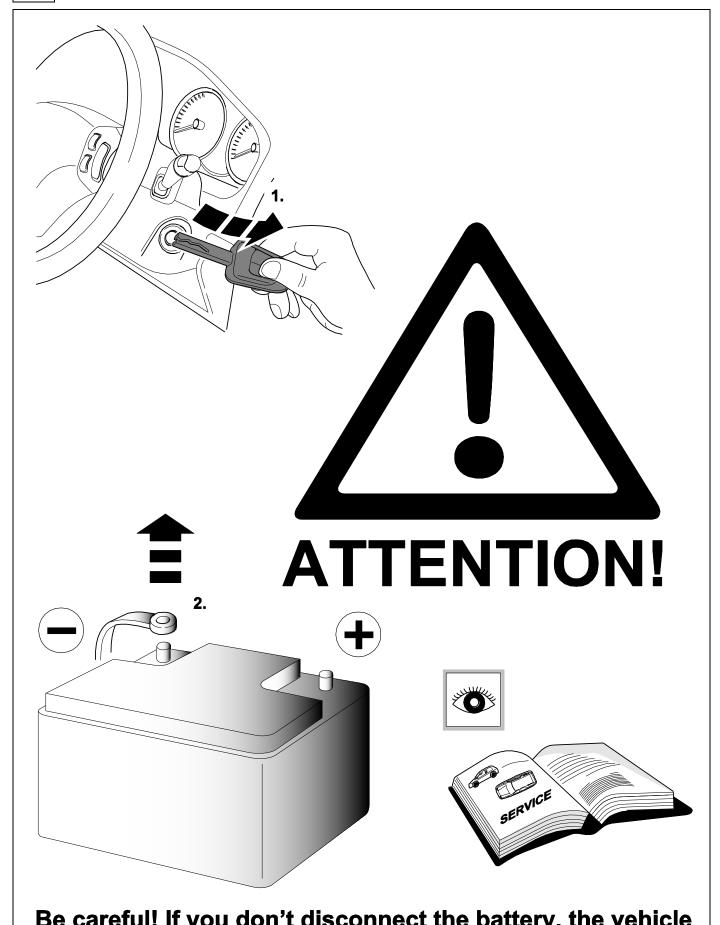
Be careful! If you don't disconnect the battery, the vehicle will show a lot of error messages in instrument panel!
