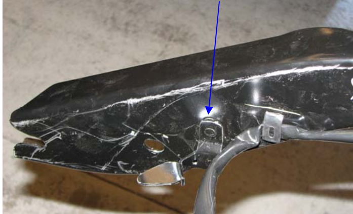
FIG 4: SHOWS THE MOUNTING BRACKET FOR THE STEP THAT NEEDS TO BE DISCARDED & REPLACED WITH THE MOUNTING BRACKET PROVIDED IN THE KIT, ON BOTH SIDES OF THE STEP.
