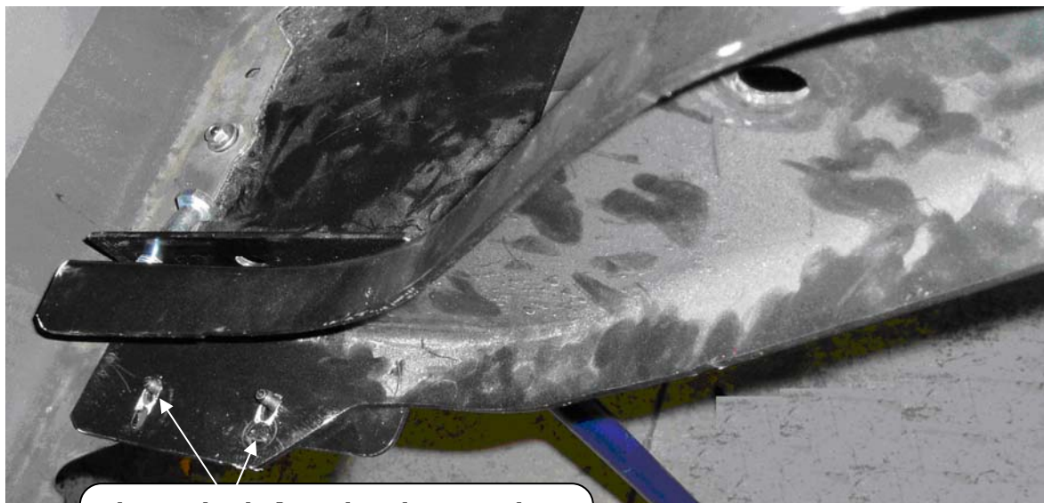
FIG 2: SHOWS BOLT HOLES THAT NEED TO BE SLOTTED.
