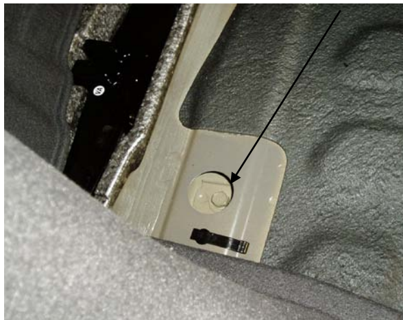
Fig 10: Remove & discard impact beam shown.
