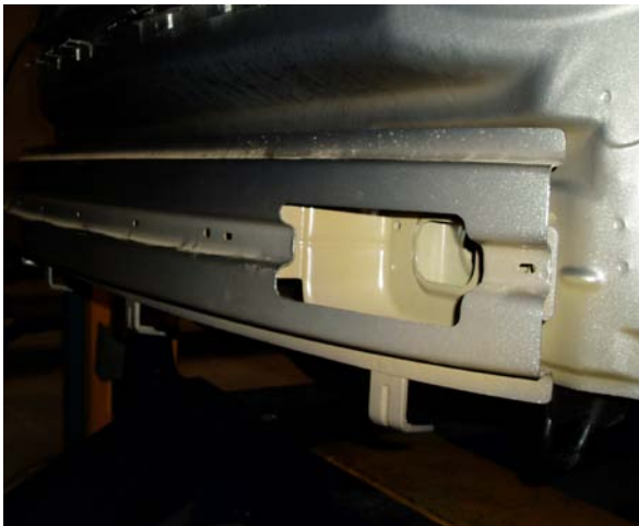
Fig 10: Remove & discard impact beam shown.
