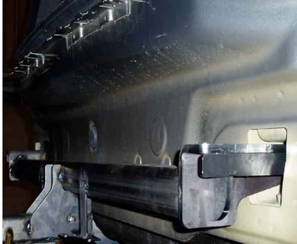
Fig 15: shows towbar mounted from inside of boot.
