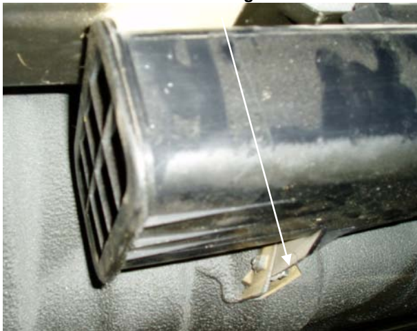
Fig 11: Remove charcoal canister, by removing bolt at the bottom of the figure shown.
