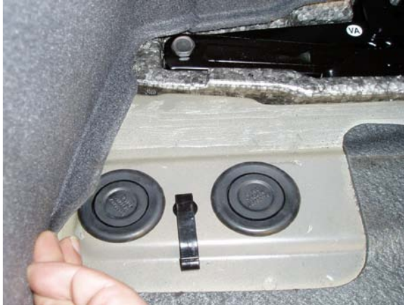
Fig 9: Remove wiring & wrap it around towbar using cable ties provided if necessary.
