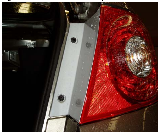
Fig 4: Two screws beside tail lamp shown.
