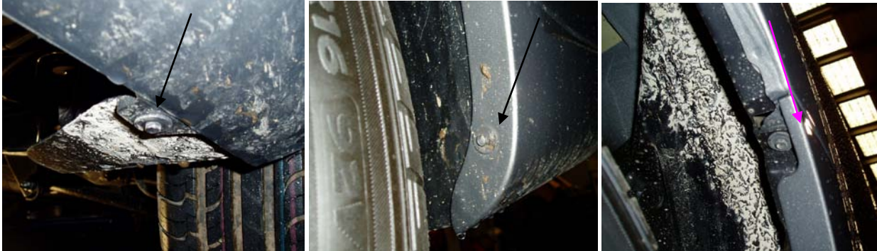
Fig 1, 2 & 3: Shows bolts that need to be removed from the side mudflaps of the vehicle
