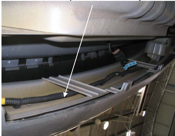
Fig 11: Remove charcoal canister, by removing bolt at the bottom of the figure shown.
