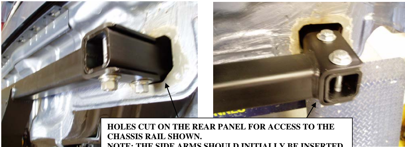
Fig 1: Shows holes cut on rear panel, side arms inserted & towbar bolted on.
