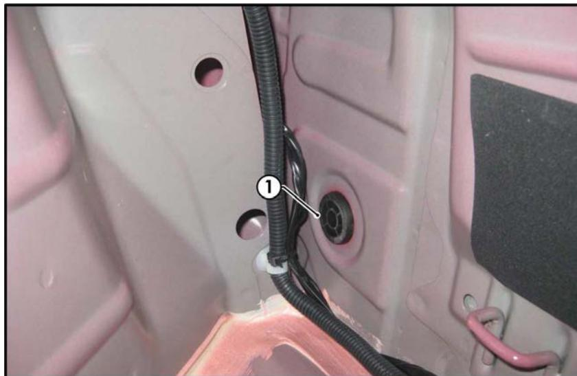
7. Drill out the grommet hole to Ø31mm.
