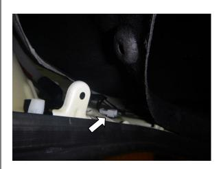
7. Remove 3x screws and 1x scrivet located inside the rear wheel well.
