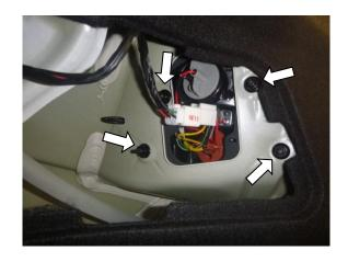
**4.** Remove 1x scrivet and 1x screw from light cavity.
