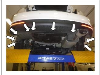
**9.** Under vehicle on LH side, remove 4x nuts and remove the tyre well protector.
