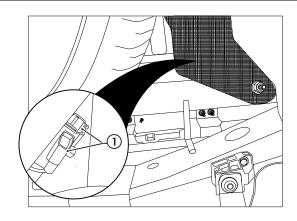
8. Connect vehicle towing 2-way and 5-way male connectors (1) to the 2-way and 5-way female connectors (2) of the trailer wiring harness as shown.
