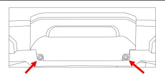
2. Push the two catches outboard to release the cover.
