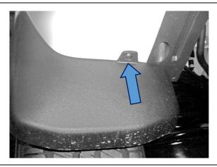
3. Remove self-tappers from wheel arch & lower skirt of bumper.
