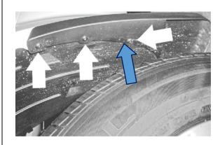
2. Remove 1 x screw from behind the mud flap and remove the mud flap.
