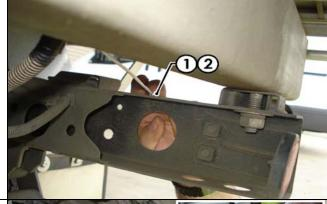
3. On the Tail Harness (tail length 1200mm) (1) and mating 8-way male connector (2), apply electrical grease or silicon on to the back of the connectors to make them water proof (3).
