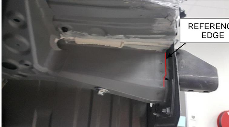
11. Insert LH side arm into chassis rail. Loosely secure with 4 x M8 bolts to vehicle rear panel complete with 1 x M8 washer per bolts.
