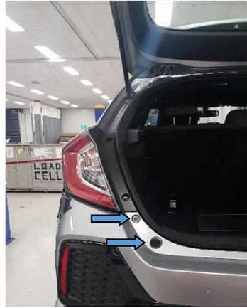
2. Remove 2 x phillips head screws from wheel arch lining on LHS.
