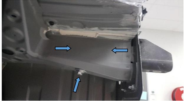
13. Lift towbar to side arms and loosely secure LHS with 2 x M10 bolts, complete with 2 x M10 washers and 1 x M10 nut per bolt.
