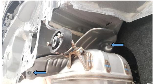
**9. Bend impact beam locating tabs down until they are in line with rear panel on LHS and RHS using a rubber mallet.**
