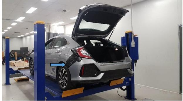
5. Remove 4 x bolts retaining impact beam on LHS.
