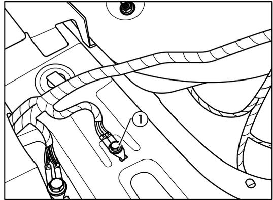
31. Route the orange power wire towards the vehicle interior Fuse box.
