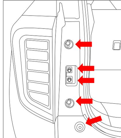
3. In wheel arch, remove 3 x screws.
