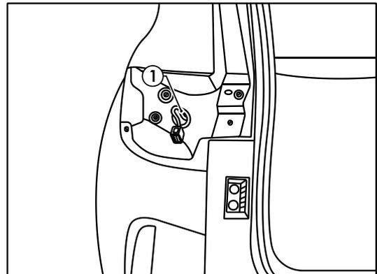
27. Behind the LHS rear panel, clean ECU mounting location (1) shown and base of ECU (2) using supplied cleaning pad.
