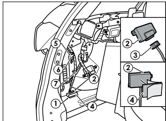
30. In the rear Cabin Area, connect the white M6 ground wire ring terminal to the vehicle earthing point **(1)** on the rear arch.
