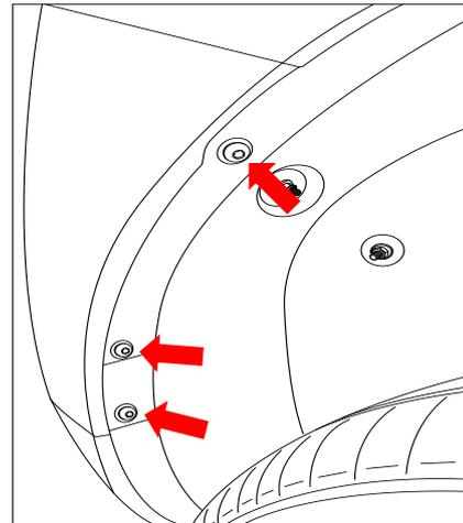
4. From under the vehicle, remove 1 x scrivet from the bumper.
