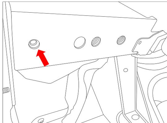
9. Position the towbar up to the chassis rail and loosely secure with 2 x M14 bolts complete with 1 x washer per bolt.
