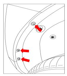
From under the vehicle, remove 1 x scrivet from the bumper.
