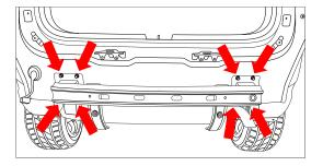
8. Enlarge the rear chassis rail mounting hole to accommodate a M12 bolt (Drill hole to 13mm). Deburr and apply an anti-corrosive coating to the exposed area.
