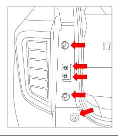
3. In wheel arch, remove 3 x screws. Repeat for other side.
