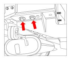
10. Secure the (drilled out) rear most hole position with 1 x M12 bolt complete with 1 x fitting plate, 2 x washers and 1 x nut. Ensure that the fitting plate is on the inside of the chassis rail.
