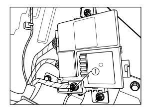
34. On the LHS of the vehicle remove the existing grommet (1) and drill out the hole to 30mm.
