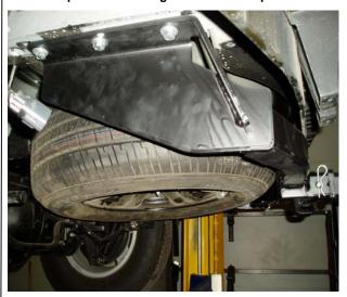
FIG 4: Shows the removed bracket being mounted back onto the vehicle on top of the towbar sidearm.
