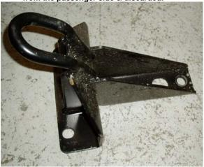
FIG 2: Shows Bracket that needs to be removed from the passenger side & tab needs to be cut off.
