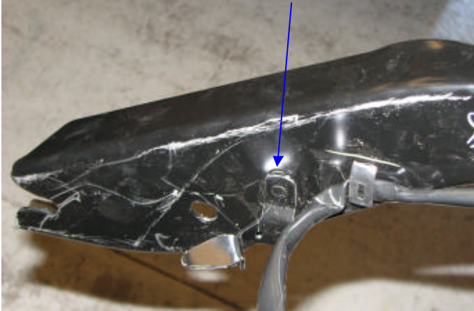
FIG 4: SHOWS THE BRACKET THAT SHOULD BE REMOVED FROM PASSENGER SIDE ARM OF BUMPER BAR.
