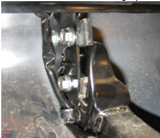
FIG 2: Passenger side arm of bumper step which has to be moved out using a packer.
