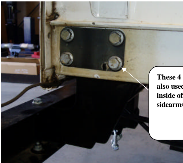
Fig 2 : Bolts used to mount the towbar shown.
