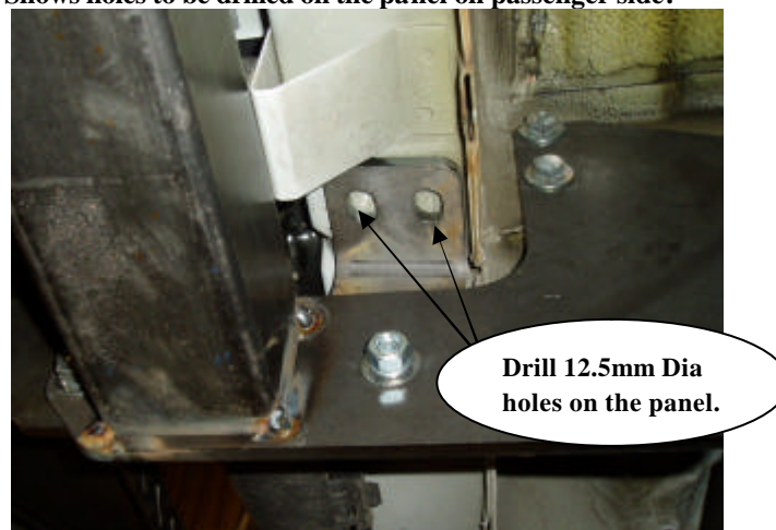
Fig 2: Shows holes to be drilled on the panel on passenger side.
