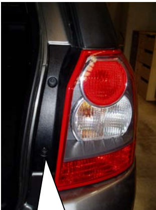
Figs 1 remove taillight assembly.
