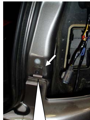
Figs 3 remove torx screws
