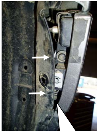
Figs 2 remove torx screws
