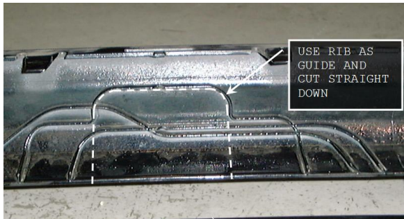
Figure 1 – Bumper cut out illustration for Sedan.
