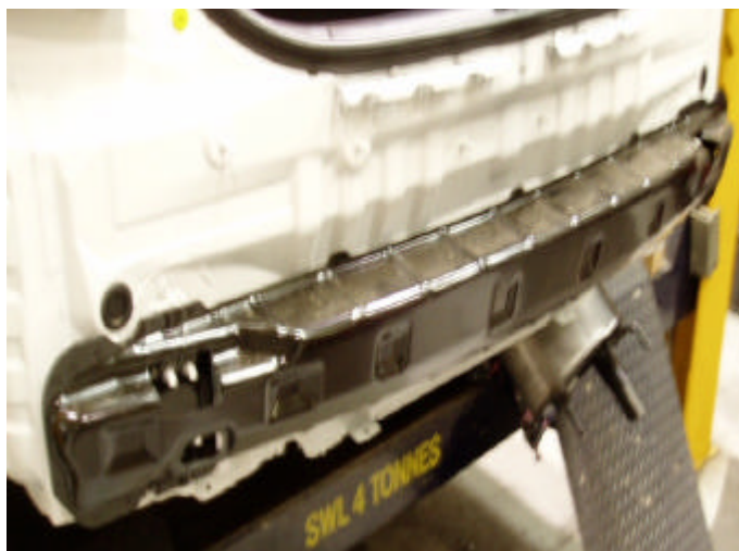
FIG 2: Shows impact beam on car
