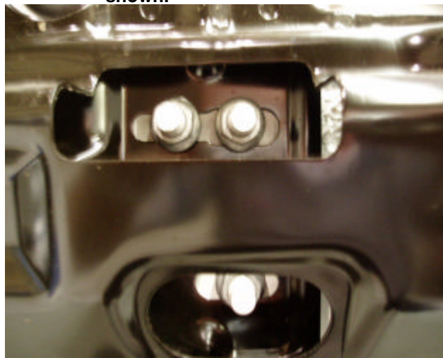
FIG 3: Discard impact beam, but retain nuts shown.
